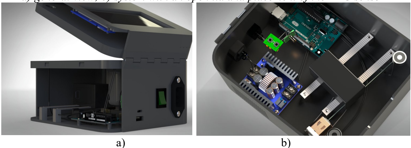
Fig. 2. Visualization of an automated system: a) controls; b) material collection system and scanning unit
