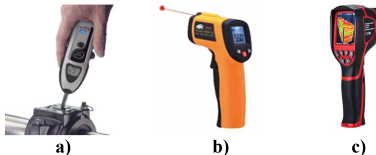
Figure 1 - Measuring instruments for monitoring the operating temperature of bearings
