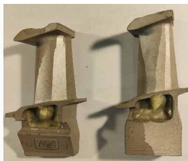
Figure 3 - Casting of blades obtained by the HSDC method
