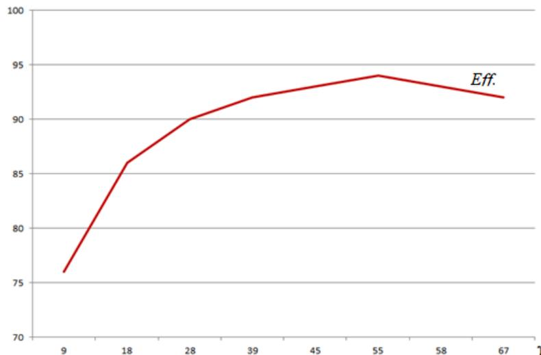
**Fig. 7 – Engine efficiency depending on the angle  $\gamma$**
