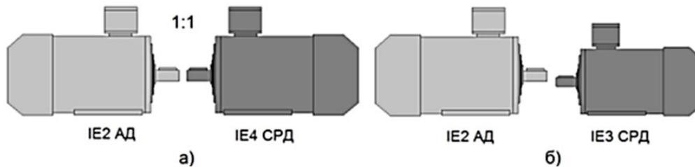
**Fig. 1 - Comparison of energy and dimensional parameters of IM and SRM of the same capacities** a) IM and high-efficiency SRM b) IM and small-sized SRM
