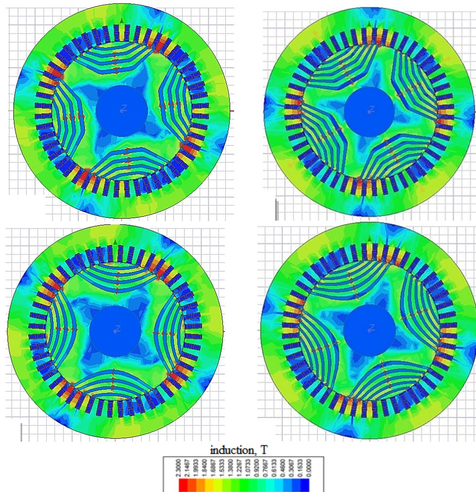
**Fig. 3 - Investigated variants of SRM rotors with definition of induction in the nominal mode of operation**
