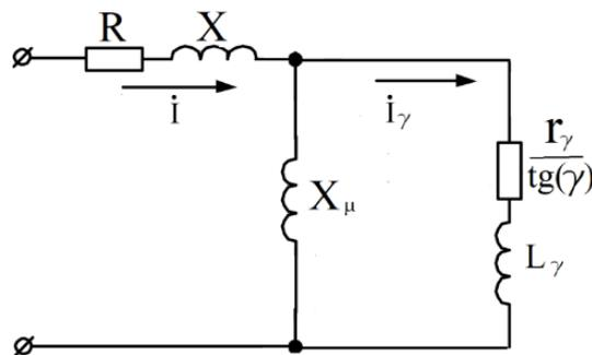
**Fig.5 - Scheme of substitution of SRM with parameters depending on the angle  $\gamma$**
