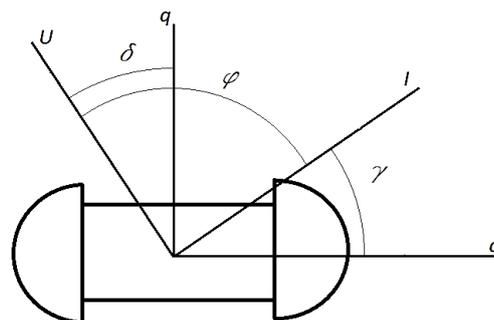
**Fig. 2 - Determination of the ratio between angles  $\phi$ ,  $\delta$ , and  $\gamma$**
