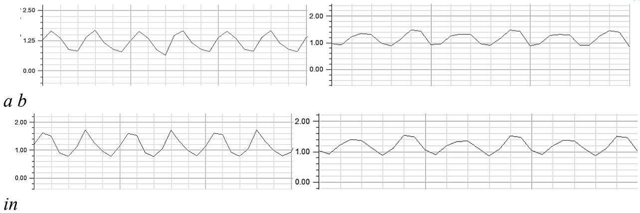
**Fig. 4 - The value of the torque on the SRM shaft and pulsations for the four tested rotor variants.**
