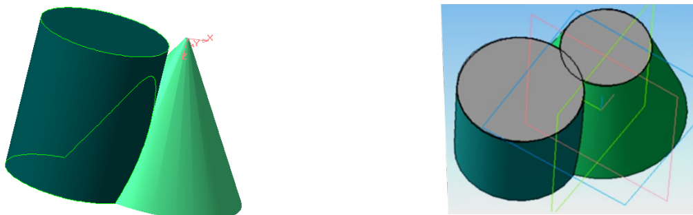
Figure 2 – 3D model (intersection of cylinder and cone)
